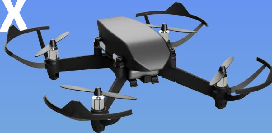
Pluto X is ideal to learn drones. Pluto, with its HD (720p) wifi camera can take photos and videos which can be used for image processing. You can program Pluto X very easily to implement using very few lines of code with its APIs.
